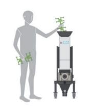
The waste is manually pulverized by putting it into granulators.
