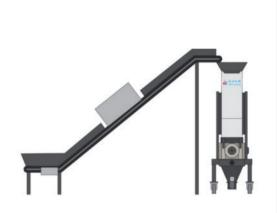
The waste material is metered and conveyed into the pulverizer by a conveyor belt for pulverization.
